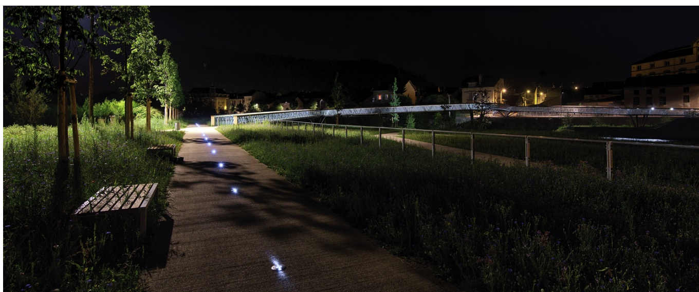
Riverside promenade. Visual delineation of the centre of the cycle path and pedestrian promenade in the City of Raon L'Etape. ECO-143 embedded solar stud (bidirectional beaconing, 1 constant white LED per side). Lighting design: Scène Publique, Agathe Argod assisted by Flore Siesling Photography: Michel Denancé.
